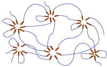
GT-730 polymer is composed of hydrophobic segment and hydrophilic segment. It forms micelles like a flower in water.
