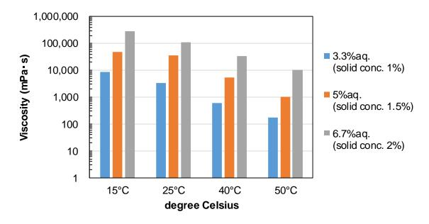
The viscosity changes reversibly by temperature in  $15 - 50^{\circ}$ C.
